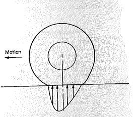
Fig. 3—Elastic wheel (rubber tire) rolling on rigid ground. Pressure distribution in the tire footprint is asymetric. Contraction of the tire periphery gives the effect of tire slip.
