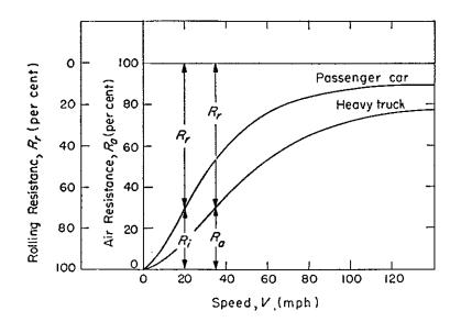
heavy truck. Considering the cruising speed on modern highways as 70 mph, it is found that an average passenger car will use 80 per cent of its tractive force to overcome air resistance. The necessity for aerodynamic perfection, especially on small cars operated at high speeds, is evident.
