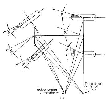
Fig. 28—Actual center of rotation of a vehicle negotiating a curve falls ahead of the theoretical center because of differences in slip angles of front and rear wheels. The cornering force, however, creates a steer-angle increasing torque, resulting usually in inherent instability of the rear-axle steered vehicle. Negative caster angle may be applied in such cases, reversing the rotation sense of the cornering force around the king pin.
