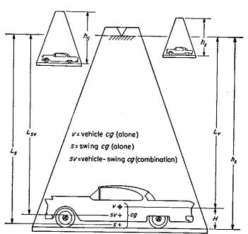
Fig. 54—Determination of center-of-gravity height by the pendulum method. Two "swing" structures (heights  $b_g$  and  $b_a$ ) are used, and the oscillation time of each is measured with the vehicle on the platform. With all other pendulum data known, cg height can be calculated.
