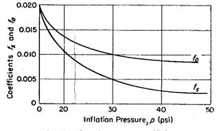
Fig. 40—Supplementary coefficients  $f_0$  and  $f_*$  for use in Equation 57.
