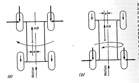
Fig. 5-Direction stability of a vehicle with four-wheel brakes. In a, rear wheels are locked, resulting in disappearance of the side-force reaction on the rear axle. Inertia force of the vehicle acts as a pushing force, and any asymetrical weight distribution (distance e) creates a self-increasing turning or skidding moment. In b, front wheels are locked. Inertia force acts as a pulling force with selfstabilizing effect.
