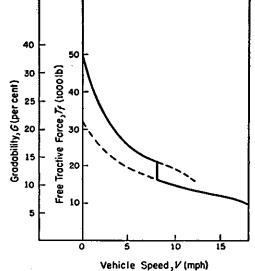
Fig. 75—Tractive force and gradability for the passenger-car example. Free tractive force  $T_i$  is obtained by subtracting motion-resisting forces from the gross tractive force T which corresponds to engine effective torque output. Gradability is proportional to free tractive force and therefore can be represented on the same diagram by recalculating the scale.
