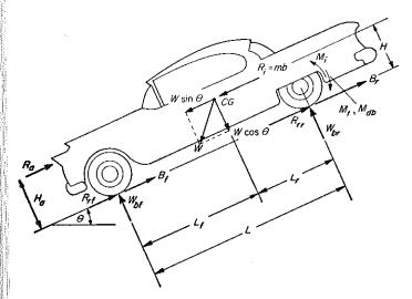
Fig. 62—Forces acting on a vehicle in decelerated motion downhill.
