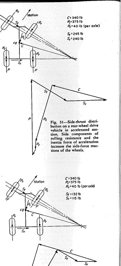
Fig. 32—Side-thrust distribution on a front-wheel drive vehicle in accelerated motion. Traction forces acting in the rolling direction of the steered wheels considerably decrease total side thrust.
