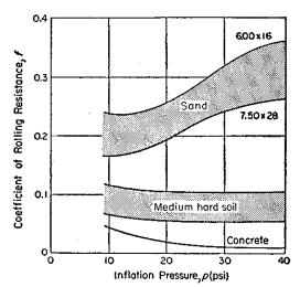
Fig. 37—Coefficient of rolling resistance as a function of inflation pressure. Values plotted assume reasonable vehicle speeds for each surface type.
