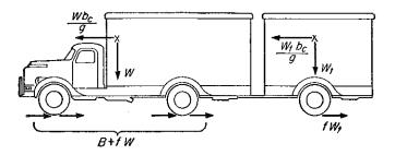
Fig. 65—Forces acting on a tractor-trailer rig when braking is provided by tractor only.
