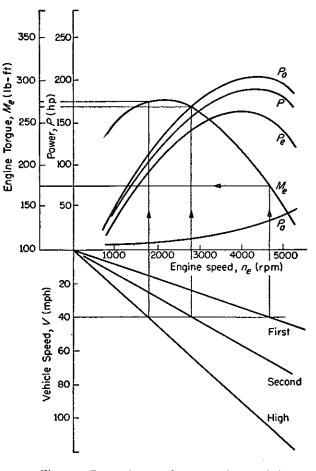
Fig. 73—Powerplant performance characteristics assumed for the passenger-car example. Upper plot shows method for obtaining effective power output  $P_{\bullet}$  from SAE standard power  $P_{\bullet}$ . Lower plot gives relationship between engine speed  $n_{\bullet}$  and vehicle speed V in first, second and high gears.
