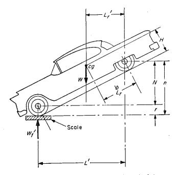
Fig. 52—Height of the cg can be determined by weighing one axle with the other elevated to arbitrary height n. With longitudinal cg position  $L_r$ known,  $L_r'$  is calculated from Equation 95. This allows two lines to be drawn that intersect at the vehicle cg. Height H can be scaled from the layout.
