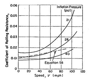
Fig. 39—Coefficient of rolling resistance as a function of speed. The effect of speed is more pronounced at lower inflation pressures. Curves for pressures of 21, 28 and 40 psi were calculated from Equation 57. An approximation for common passenger car speeds and inflation pressures is given by the plot of Equation 58.
