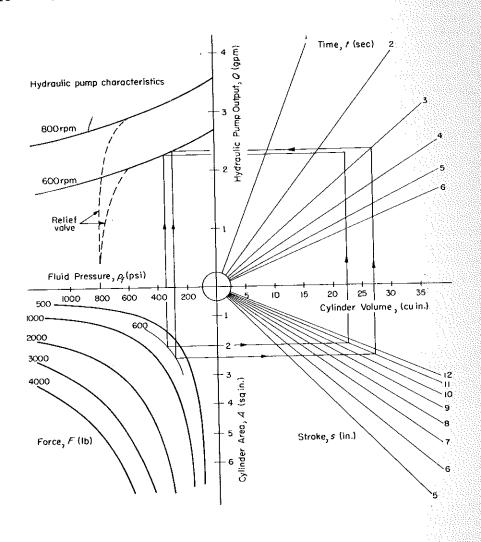
Fig. 26—Power-steering calculation chart, representing E q u ations 27 and 28. Pump characteristics are approximate and can be replaced by exact values if desired.
