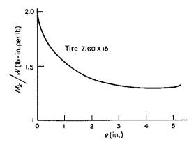
Fig. 18-Static-steering torque per unit radial load as a function of king-pin offset.
