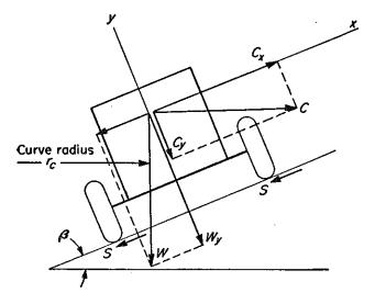
Fig. 33—Balance of forces on a vehicle negotiating a superelevated (banked) curve. Vehicle will slide to the outside of the curve if the resultant of forces acting in the x direction exceeds the maximum frictional sideforce reaction.
