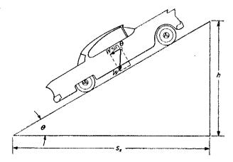
Fig. 41—Grade resistance of a vehicle is the downhill component of its weight. Grade is usually measured in per cent where  $G(\%) = (100 \ b)/s_x = 100 \ \tan \theta$ .
