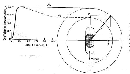
Fig. 4—Coefficient of road adhesion as a function of tire slip. Maximum ordinate value—static coefficient  $\mu_0$ —is reached between 10 and 20 per cent slip. Higher angles result in an unstable condition, with tire action rapidly changing to pure
