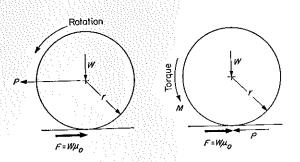
Fig. 1—Tractive force on a rolling wheel can be an external towing force (left) or result from an internally developed torque (right). Rolling continues as long as the tractive force remains within limits of the static-friction force.
