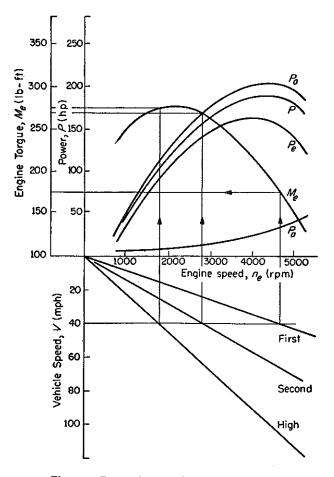
Fig. 73—Powerplant performance characteristics assumed for the passenger-car example. Upper plot shows method for obtaining effective power output  $P_o$  from SAE standard power  $P_o$ . Lower plot gives relationship between engine speed  $n_o$  and vehicle speed V in first, second and high gears.
