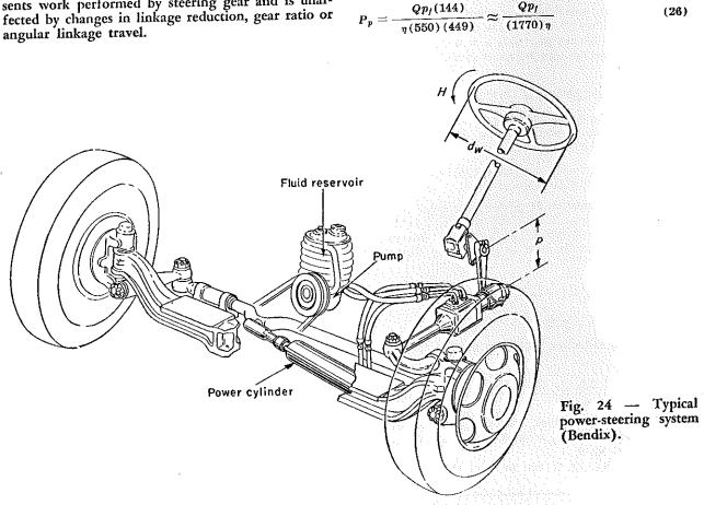
where  $P_p$  = power required (hp), Q = volume output (gpm),  $p_f$  = pressure (psi) and  $\eta$  = total efficiency of the pump (usually 70 to 80 per cent). Characteristic curves supplied by pump manufacturers showing the relation between Q and p for different pump speeds are, in practical applications, cften distorted by use of flow-control and relief valves. It is therefore advisable to find actual pump output by experiment.
