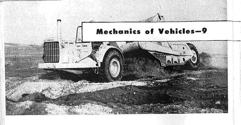
AXIMUM transferable tractive force—as determined by the nature of the wheel-ground connection—sets a fundamental limit to vehicle performance. It follows, therefore, that the type of drive employed in the vehicle—front, rear, or four-wheel—influences its ultimate capacity for speed, acceleration, gradability, and drawbar pull.
