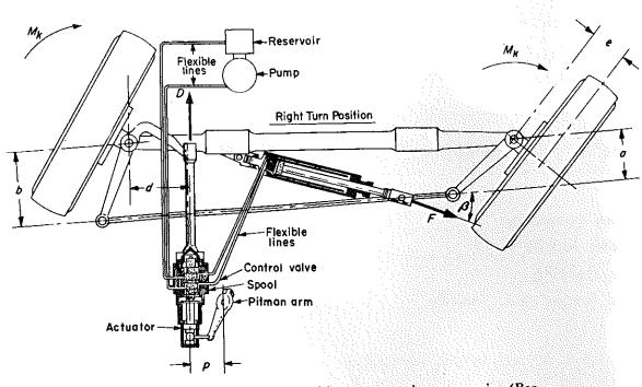
Fig. 21—Spindle-lever linkage with power-steering accessories (Bendix). If handforce applied to the steering wheel exceeds the force required to operate the control valve, the manual-steering force supports efforts of the power cylinder.
