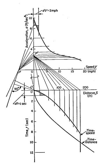
Fig. 79—Construction of time-speed and time-distance curves for the truck example. Techniques are the same as those used in construction of Fig. 77. Acceleration values in this case do not reach zero since maximum engine speed is limited by an engine governor.
