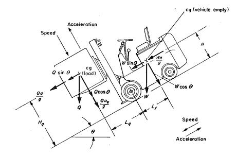
Fig. 56—The fork lift truck is representative of vehicles designed to carry loads outside of their wheelbases. The sketch illustrates the stabilityaffecting factors for the general case: downhill slope, deceleration of the vehicle in translatory motion and deceleration of the load while being lowered. STATIC STABILITY ON LEVEL GROUND: The rearranged stability equation is
