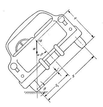
Fig. 51—By tilting the vehicle to one side until it balances, vertical height of the cg can be calculated from a measurement of tilt  $\beta$ . This method of locating the cg requires that front and rear wheels have the same tread.
