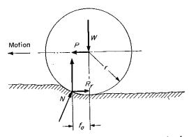
Fig. 2—Rigid wheel rolling on plastic ground. Coefficient of rolling resistance  $f_o$  has the dimension of length.
