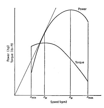
Fig. 70—Typical full-throttle characteristics of a gasoline engine. Maximum torque is given at speed  $n_{M}$ , which corresponds to the point of tangency of a line drawn from the origin to the power curve. Minimum speed,  $n_{min}$ , is engine idling speed; maximum torque is reached at relatively low power levels. Both of these characteristics account for the poor adaptability of the internal combustion engine for vehicle propulsion and point up the need for a change-gear transmission.
