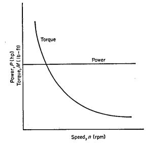
Fig. 68—Powerplant characteristics ideally suited for vehicle propulsion show constant power output over the entire speed range. This gives a hyperbolic torque curve and provides high tractive forces for vehicle acceleration at low road speeds. vehicle powerplant are introduced, and methods for correcting standard data to existing atmospheric conditions are reviewed. Also surveyed are the power losses in accessories and drive-system components.
