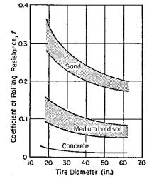
Fig. 38—Coefficient of rolling resistance as a function of tire diameter. Effect of tire diameter is negligible for hard surfaces (concrete) but decisive for soft ground or sand.
