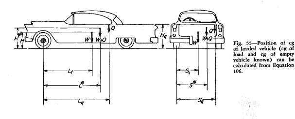
the vehicle cg, is not given here. Form of the equation, where cap and lower-case subscripts refer to the long and short swings, is
