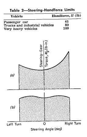
Fig. 23—Torque on gearbox output shaft as function of steering angle. An example of poor steering-gear design is shown at *a*; torque peaks on one side of straight-ahead position. Desirable torque distribution is shown at *b*. Shaded area under each curve represents work performed by steering gear and is unaffected by changes in linkage reduction, gear ratio or angular linkage travel. the usual power-steering system, Figs. 21 and 24, are described in the following sections.
