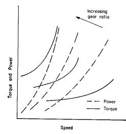
Fig. 63—Braking potential of a throttled engine. Three sets of torque and power-consumption curves show the effect of gear ratio on engine braking capacity. Quite obviously, "shifting down" helps retard the vehicle on downhill runs
