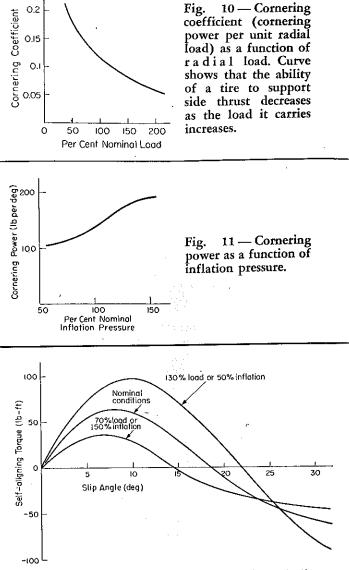
Fig. 12-Self-aligning torque as a function of slip angle. At high slip angles, self-aligning torque becomes negative, acting in a steer-angle increasing direction. Radial load and inflation pressure, because they determine footprint area, have an effect on self-aligning torque.
