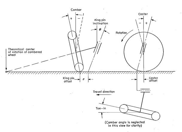
Fig. 14—Wheel orientation with the ground.
