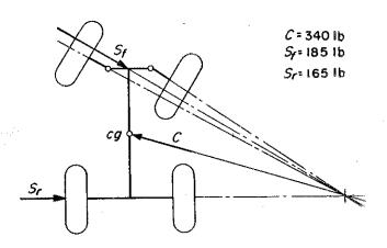
Fig. 30—Side-thrust distribution to front and rear wheels on a vehicle negotiating a curve. Only centrifugal force is assumed to act in this simplified case (rolling resistance is neglected).
