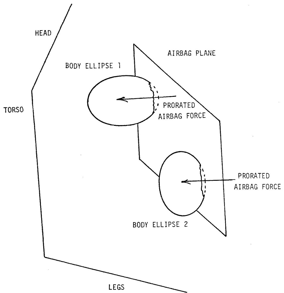
Figure 4. Application of Airbag Force
