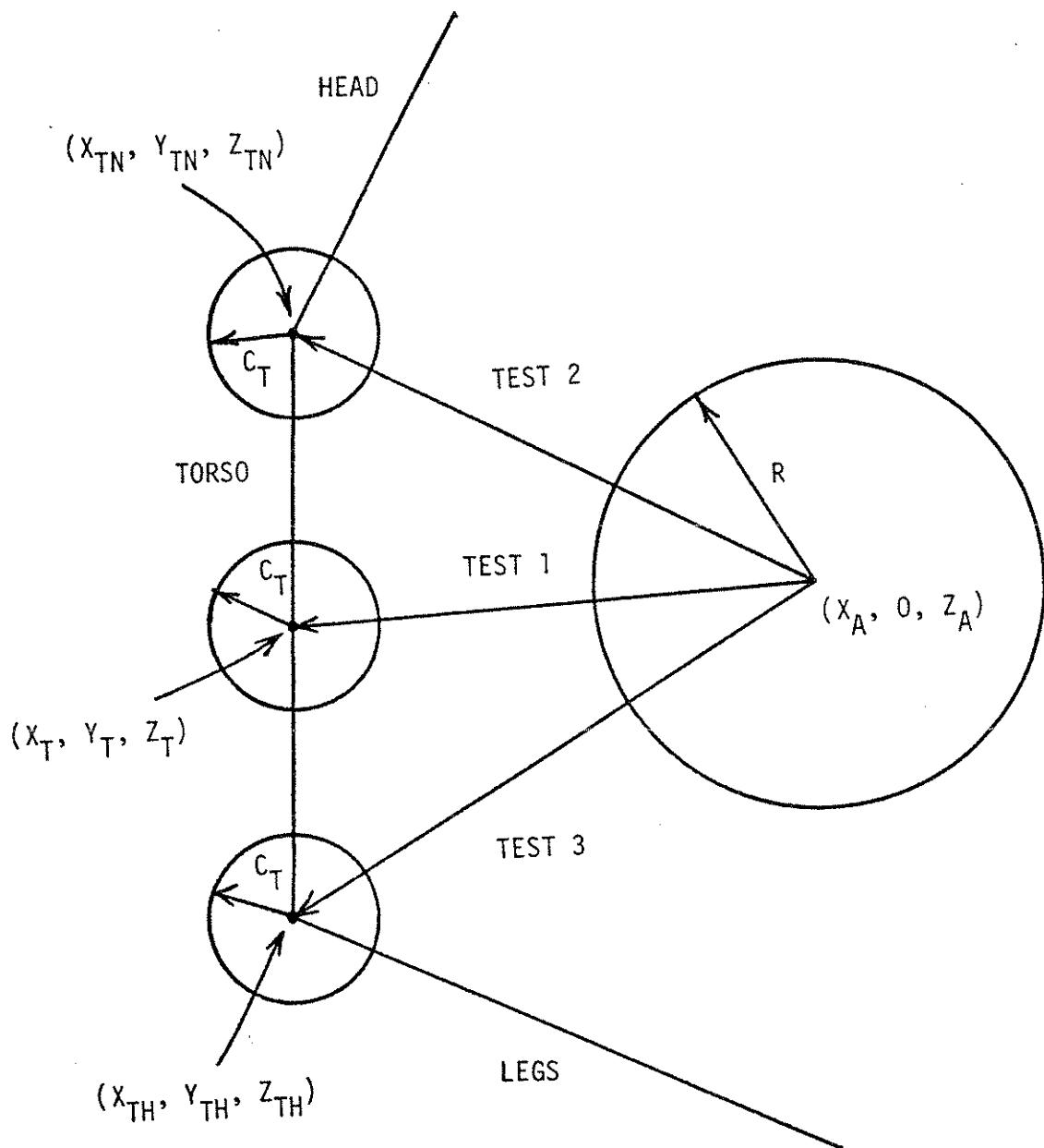
Figure 2. Testing for Occupant-Airbag Contact
