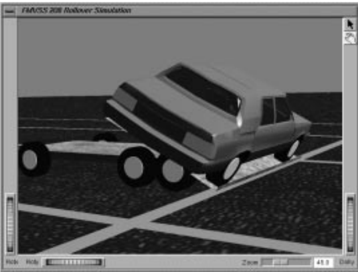
Figure 7 - FMVSS rollover test setup. The actual test setup is shown at the top [24], and the simulation setup is below.
