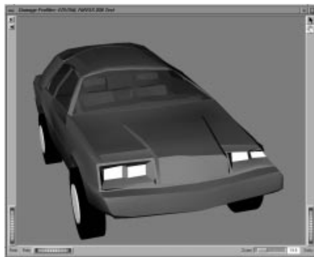
Figure 10 - Simulated vehicle damage resulting from FMVSS 208 Rollover Test.
