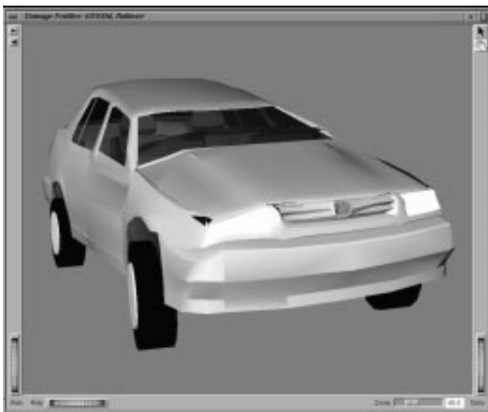
Figure 15 - Simulated vehicle damage resulting from the off-road rollover crash.
