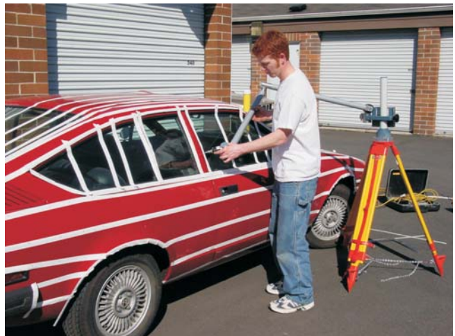
Using the FARO digitizing arm to measure the exterior of the vehicle for the geometry file.
