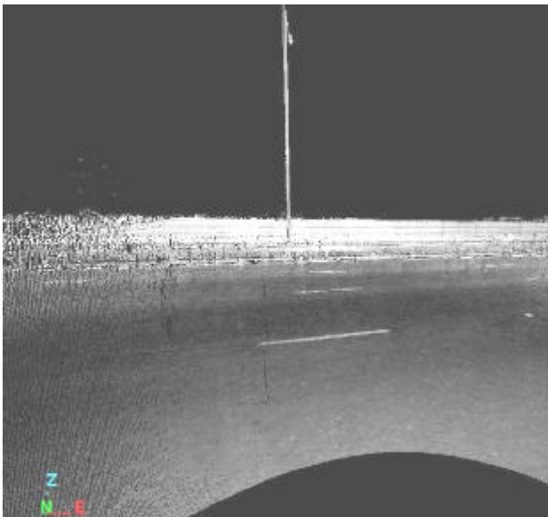
Figure 6 View of scan data from the 'scanner eye' perspective after the removal of transient data caused by vehicles
