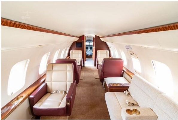
Figure 6: Business jet seating layout included both forward and aft facing seats on the left and right side of the aircraft as well as a leftward facing couch on the right side of the aircraft. All orientations were simulated.
