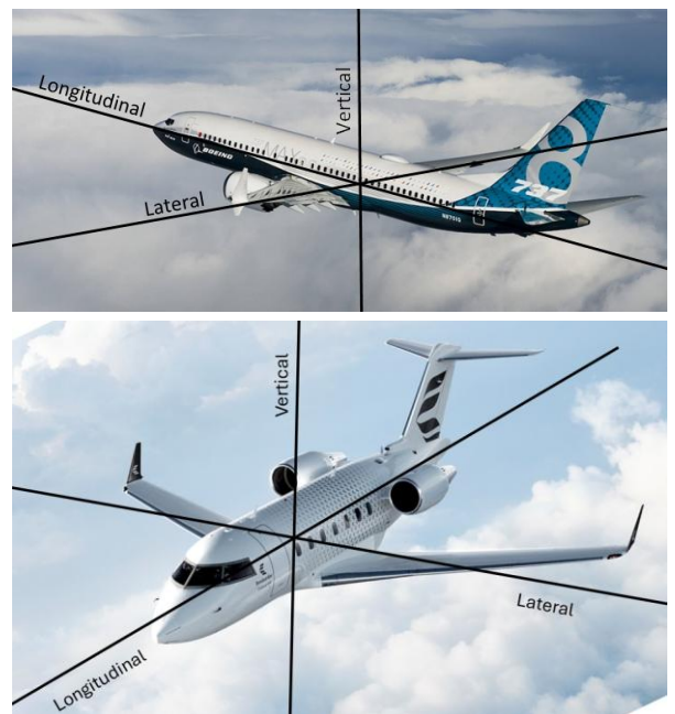
Figure 2: Examples of the two aircraft involved and the non-inertial reference frames attached to each.
