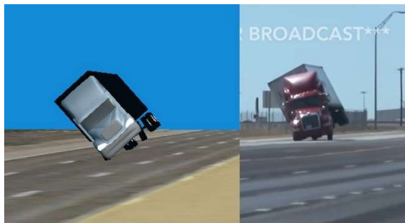
Figure 1: Comparison of unaltered SIMON simulation to a real world rollover
