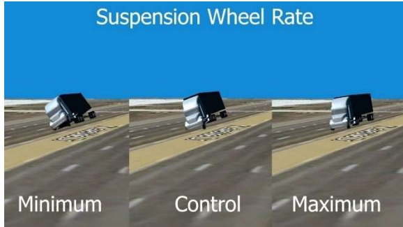
Figure 3: Wheel rate comparison at the same duration into the roll event.
