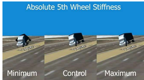
Figure 5: Comparison of the absolute 5 th wheel stiffness range
