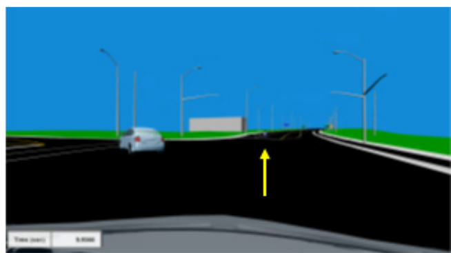
Figure 8: Using HVE to match the vehicle positions shown in the dashcam to determine vehicle speeds
