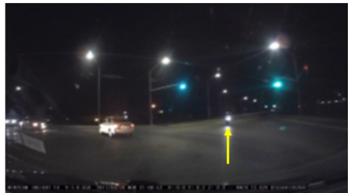
Figure 7: Traditional position vs. time analysis for other vehicles shown in dashcam footage. Shown above are two positions of an oncoming motorcycle, 1.27 seconds apart.
