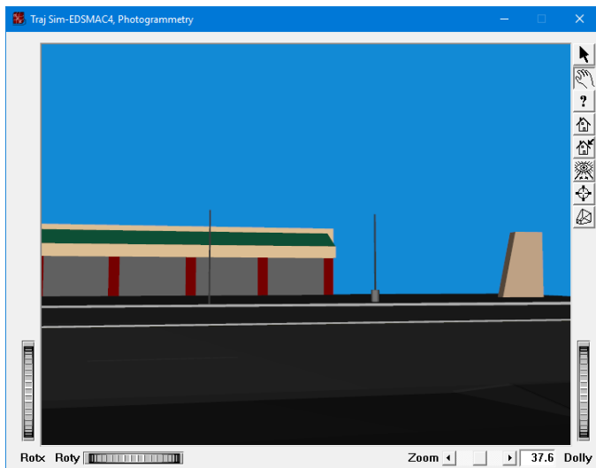
Figure 8. Three-dimensional computer model of the above site built from a total station survey. In addition to the roadway, the building, light poles and wall were located.
