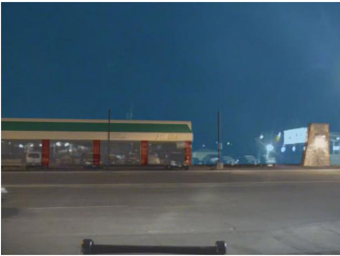
Figure 15. A Traj Sim window superimposed over an extracted frame from a dash cam video. The transparency setting was adjusted to visually evaluate the alignment of visible landmarks.
