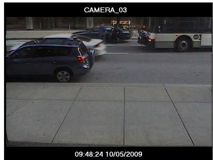
Figure 1. Letterboxed image from a surveillance video with camera, date and time information displayed in the mattes. The image was compressed vertically. It was necessary to restore the image to the original aspect ratio for photogrammetric purposes.
