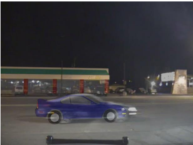
Figure 18. The Traj Sim window was superimposed over the extracted frame. The simulated vehicle is not aligned with the video. The simulation was advanced, and the process repeated.
