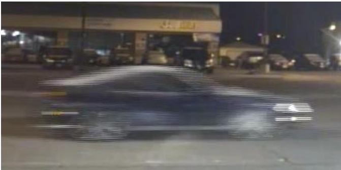
Figure 2. Interlaced video divides the image into separate fields of horizontal lines which are alternatingly refreshed. Moving objects are subject to a combing effect which affects the ability to precisely locate the object.
