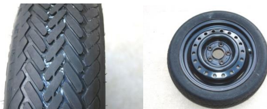
Figure 2: Goodyear T125/70-D14 space-saver spare tire
