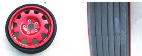
Figure 3: Vredestein 165/70-16 space-saver spare tire
