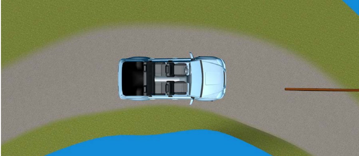
Figure 8: Vehicle traveling in the center of the road with the pole located near the center of the road.
