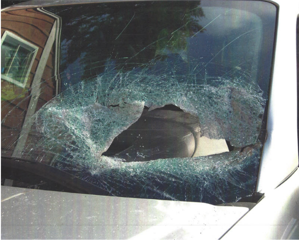
Figure 1: Impact and penetration location of pole through windshield at the driver's side A-pillar.
