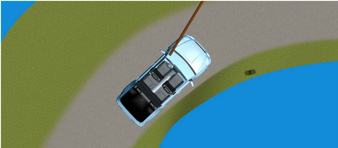
Figure 9: Pole penetrating the windshield.
