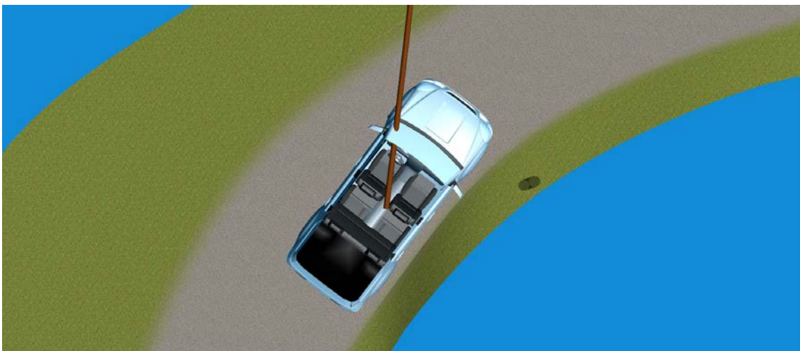
Figure 10: Pole rotating due to contact with driver's side A-pillar.
