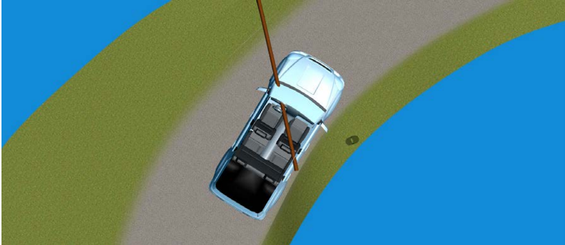
Figure 11: Pole continuing to rotate due to contact with the driver's side A-pillar and exiting the incorrect rear passenger's side window.
