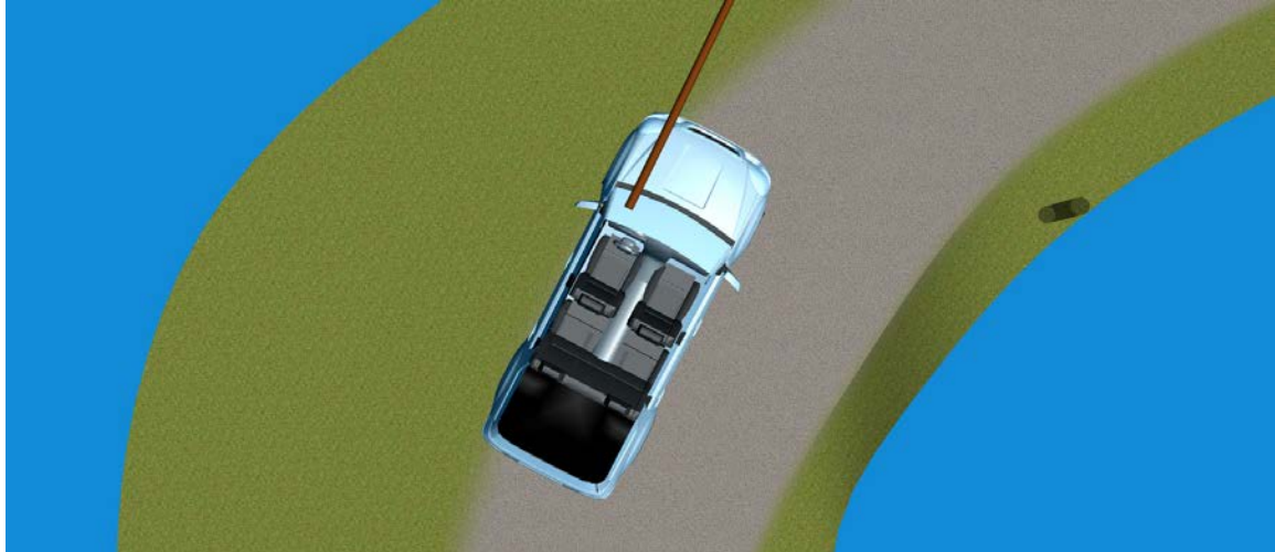
Figure 12: Vehicle traveling at the edge of the roadway with the end of the pole located off of the traveled portion of the road showing the pole penetrating the windshield.
