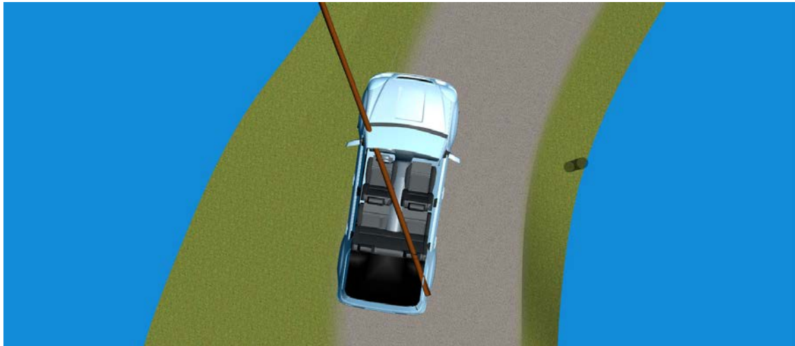
Figure 14: Pole rotates due to contact with the driver's side A-pillar to exit the rearmost passenger's side window.
