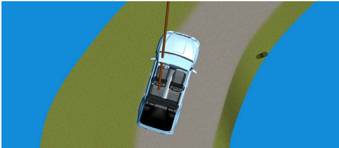
Figure 13: Pole traveling through the vehicle to impact the driver's side headrest.
