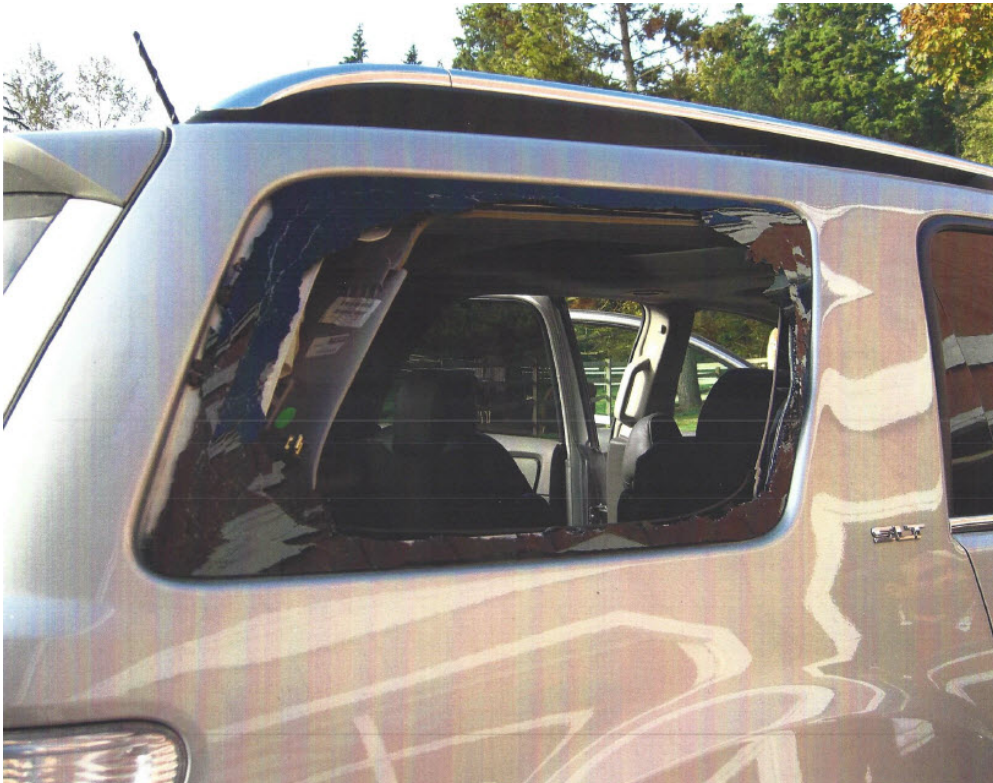
Figure 2: Pole exit location through small rearmost passenger's side window.
