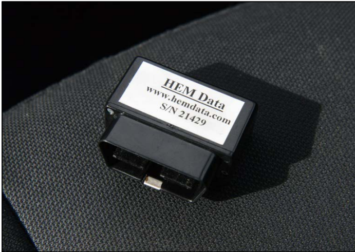
Figure 2 – “OBD Mini Logger” manufactured by HEM Data Corporation
