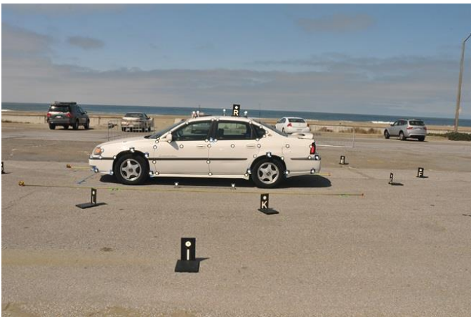
Figure 1: Photomodeler targets on Chevrolet Impala
