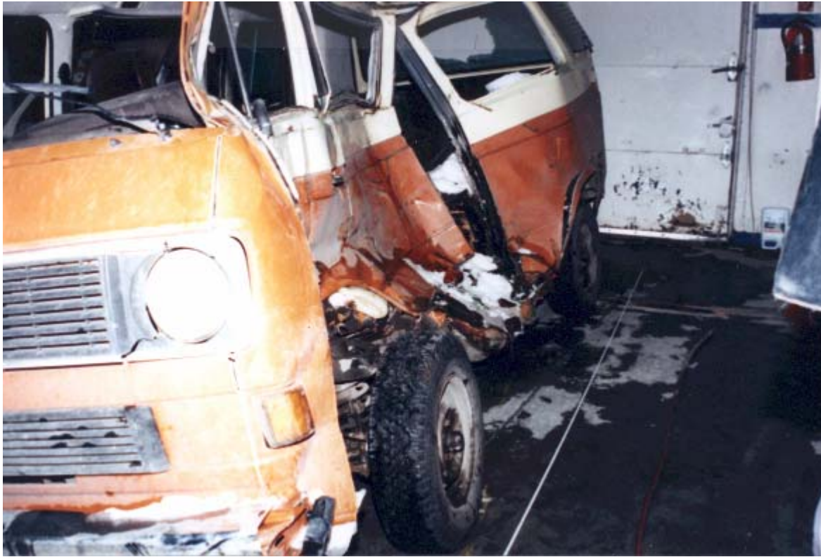
Figure 9 - View of severe impact damage on the left side of the Vanagon. Tape measure and damage outline drawn on the concrete floor are also visible.
