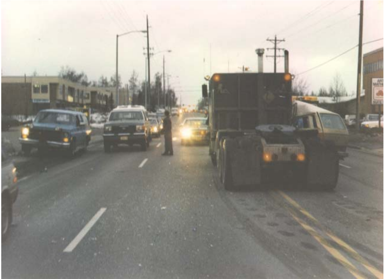
Figure 14 - Close-up view of the Peterbilt at rest. The left front tire is steered to the right, and caused a sweeping scuffmark visible in the photo. This information indicates the driver was attempting to steer back into the southbound lanes after impact.
