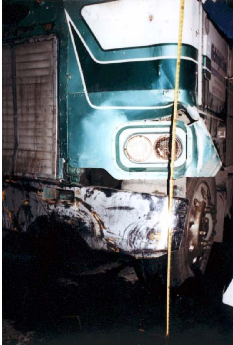
Figure 5 - Left frontal view of Peterbilt tractor shows damage to bumper and left front corner.
