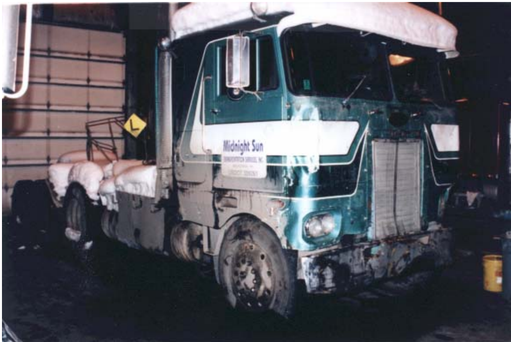
Figure 4 - Oblique view of 1975 Peterbilt tractor. Note the minor frontal damage.
