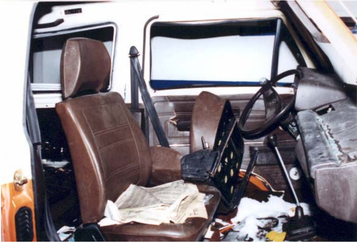
Figure 10 - View of Vanagon interior showing the driver's seat dislodged from its tracks.
