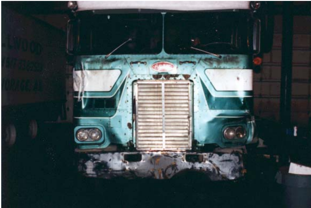
Figure 3 - Frontal view of 1975 Peterbilt tractor as inspected on January 5, 1992. Note the black, circular impression towards the left end of the bumper. This impression was caused by the Volkswagen's left front tire.
