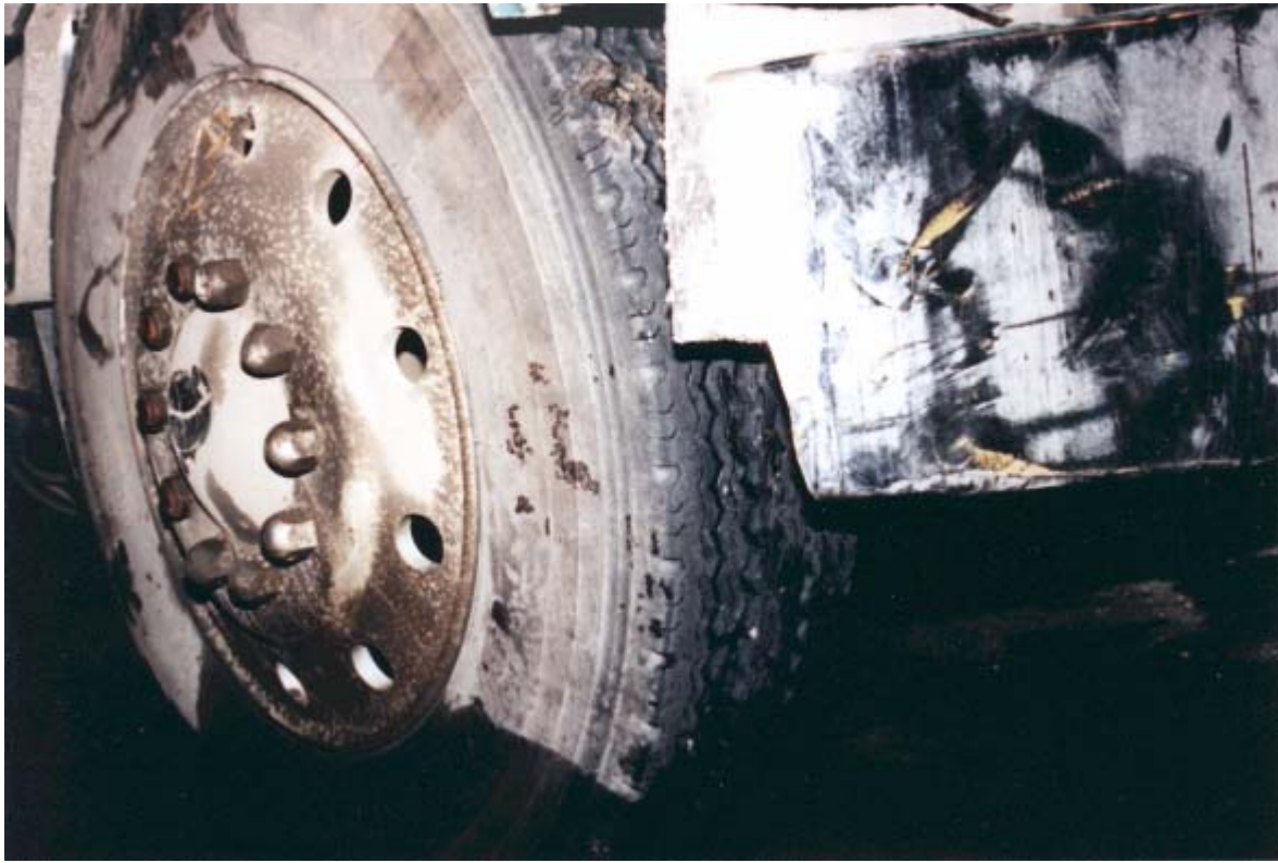
Figure 6 - Close-up view of right end of the Peterbilt bumper showing paint transfers from the Volkswagen Vanagon. The condition of the left front tire is also visible; the condition of this tire was typical of other tires on the vehicle.
