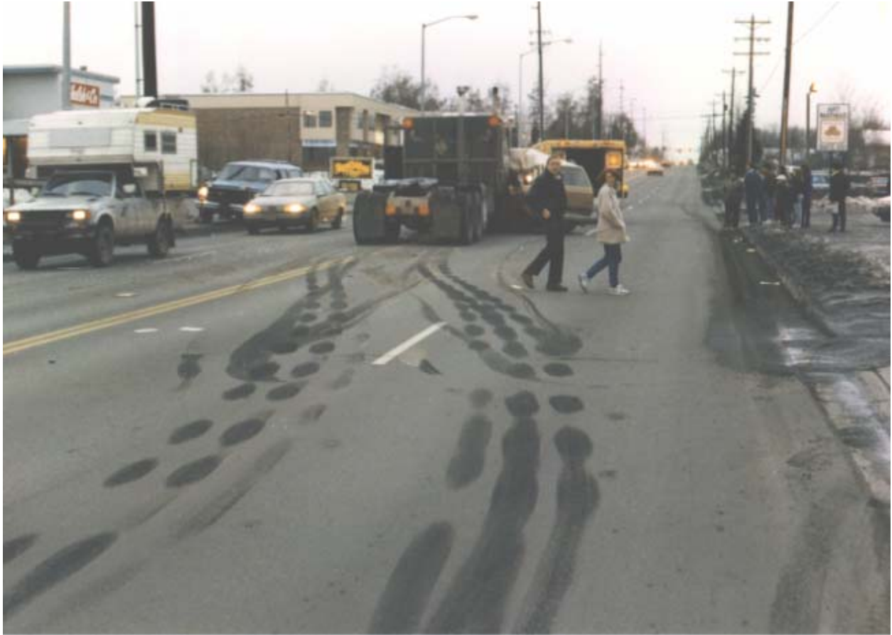
Figure 13 - Closer view of vehicle at the crash site. Note the character of the tire marks. The heavily striated marks were caused by the Vanagon's tires as it was pushed laterally. These marks identify the location of the Vanagon at impact.
