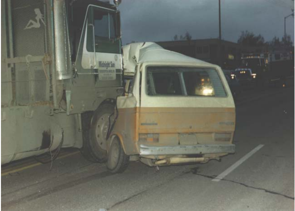
Figure 15 - Close-up of the vehicles at rest showing the severe penetration of the front of the Peterbilt tractor into the left side of the Vanagon. Note also the striated tire mark leading to the left rear tire of the Vanagon, and the thin tire mark leading to the debaded right front tire of the Vanagon.
