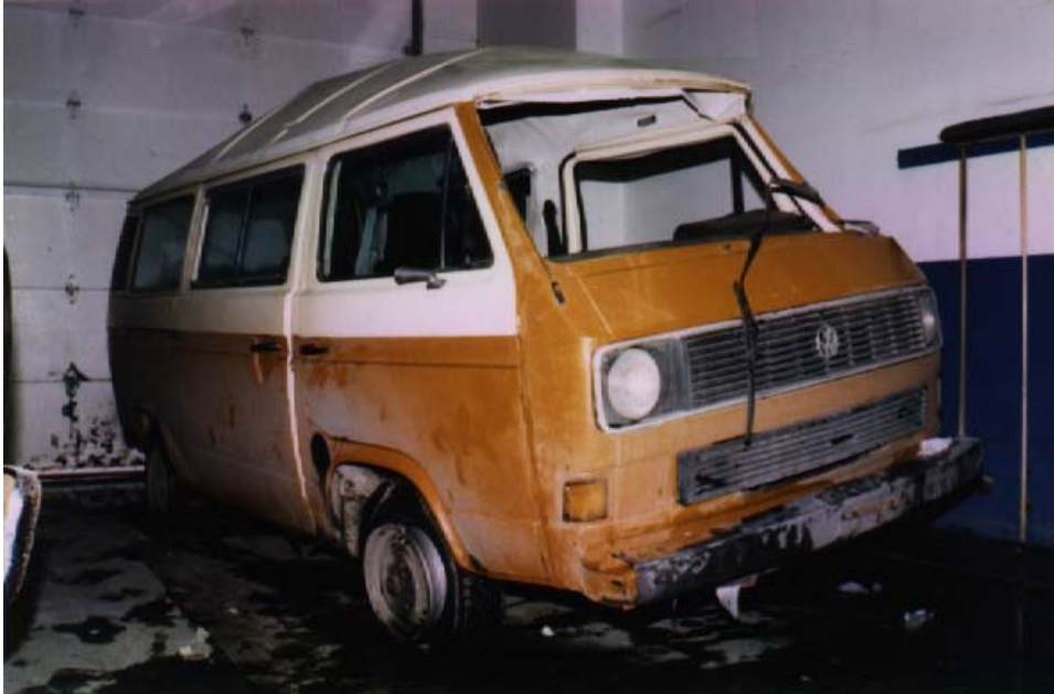
Figure 8 - Oblique view of 1982 Volkswagen Vanagon. Note that both right-side tires are debeaded and not inflated. The right front wheel rim shows evidence of lateral skidding that led to the debeading.
