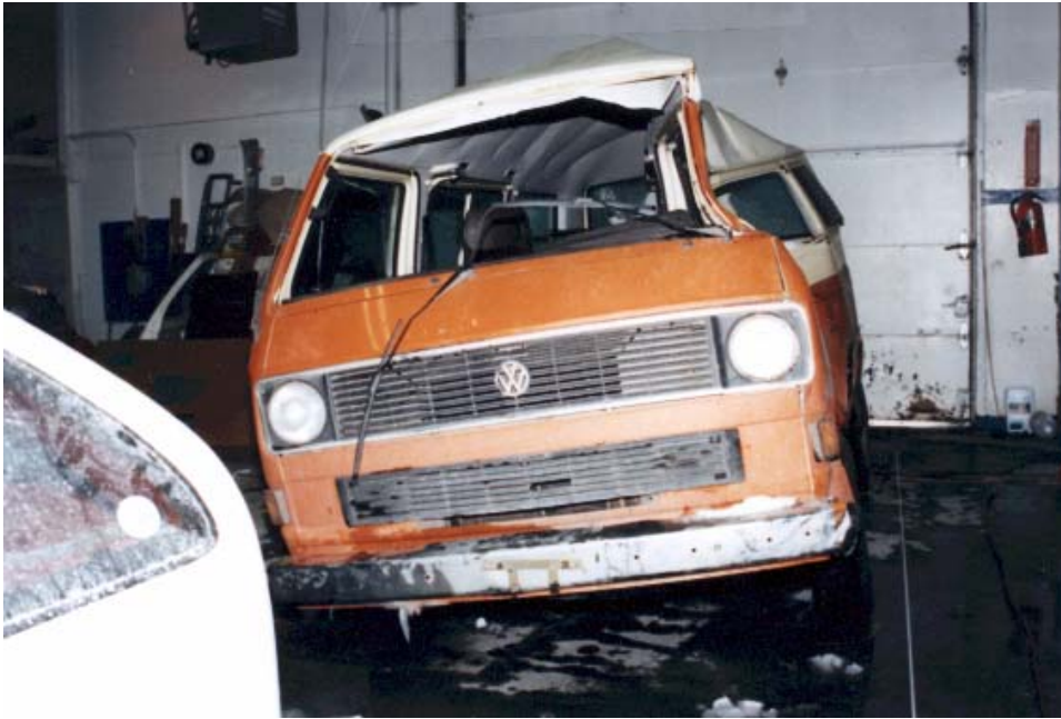
Figure 7 - Frontal view of 1982 Volkswagen Vanagon as inspected on January 5, 1992. Note severe impact damage on the left side.
