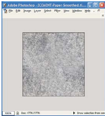
Figure 6 – Texture map after offset filter and smoothing via the Clone Stamp tool
