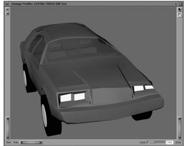
Figure 10 – Simulated vehicle damage resulting from FMVSS Rollover Test.
