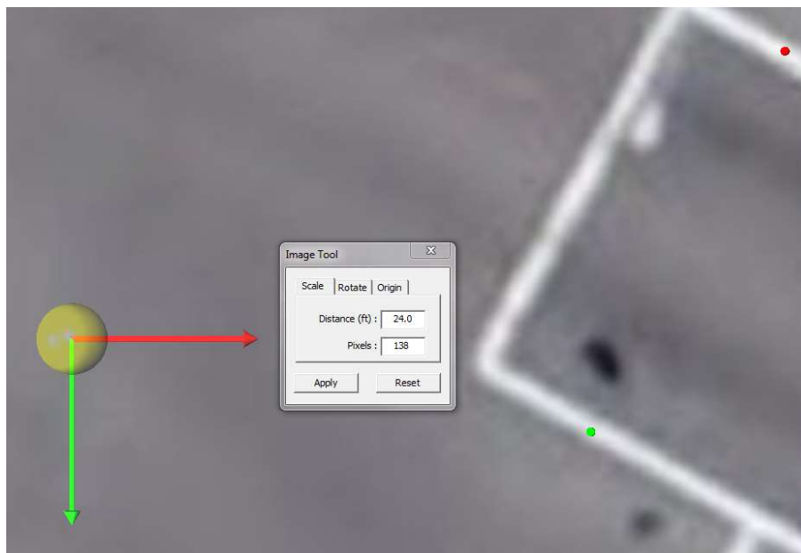
Figure 1 - Bottom portion of the Environment Information dialog, showing the current method for adding and scaling an aerial image.
