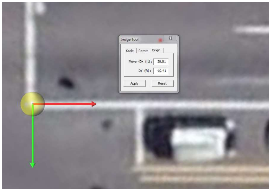
Figure 4 - The Origin Tool allows the user to move the earth-fixed origin to a new location. In this example, the origin initially in the middle of the intersection (see Figure 3) was moved to the intersection between two pavement stripes.
