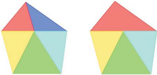
Figure 2 - Watertight mesh (left) and non-watertight mesh (right).
