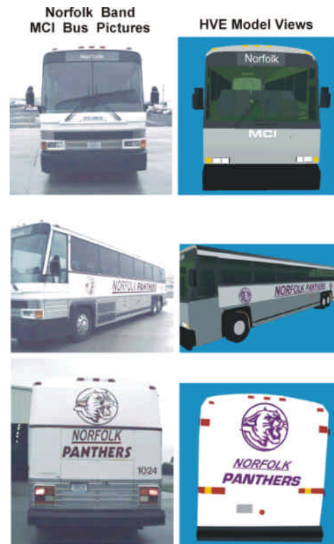
Figure 2 – Comparison of pictures of the Norfolk motor coach to the HVE model
