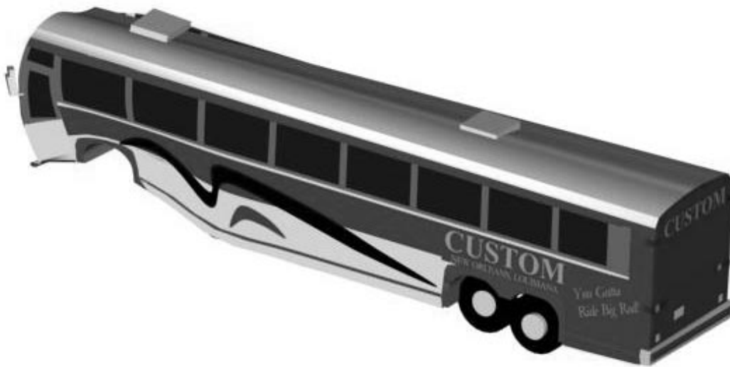
Figure 5: The three-dimensional model of the accident bus after deformation in 3D Studio Max at the final rest location
