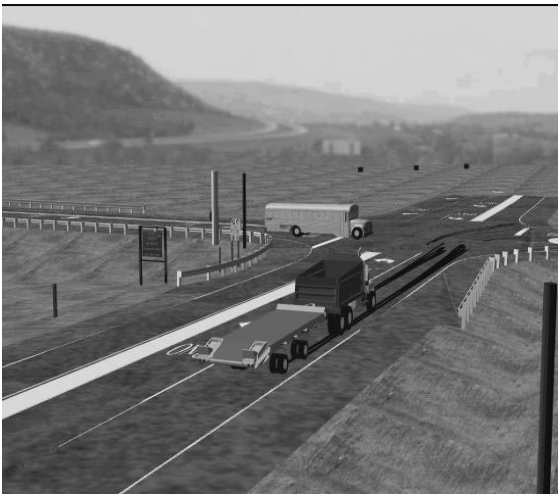
Figure 10: A single image from the Central Bridge, NY HVE simulation immediately prior to the collision between the dump truck and the school bus.
