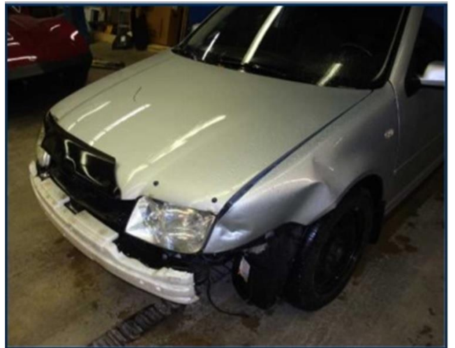
Figure 4: A view of the left front of the Volkswagen Jetta (V1) with the front bumper cover removed.
