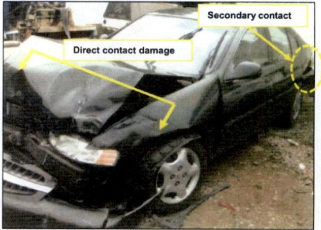
Figure 5: A view of the left front of the Nissan Altima (V3) showing primary and secondary contact damage.
