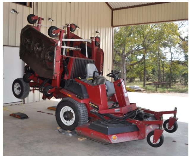
Figure 3. Center of Gravity Measurement.
