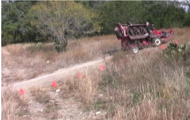
Figure 4. Test slope for determining drag factor.
