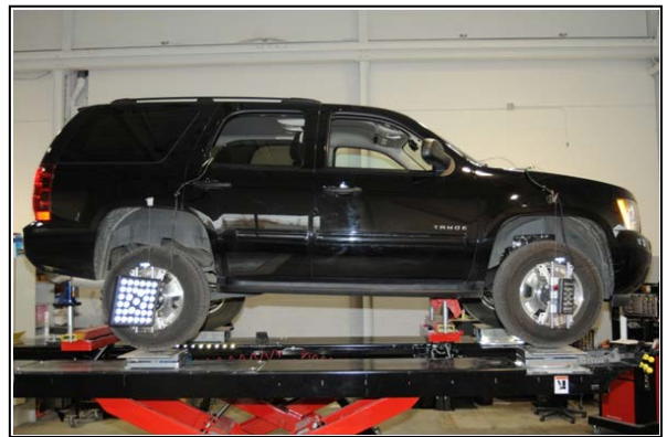
Figure 5a: Vehicle raised to full suspension travel
